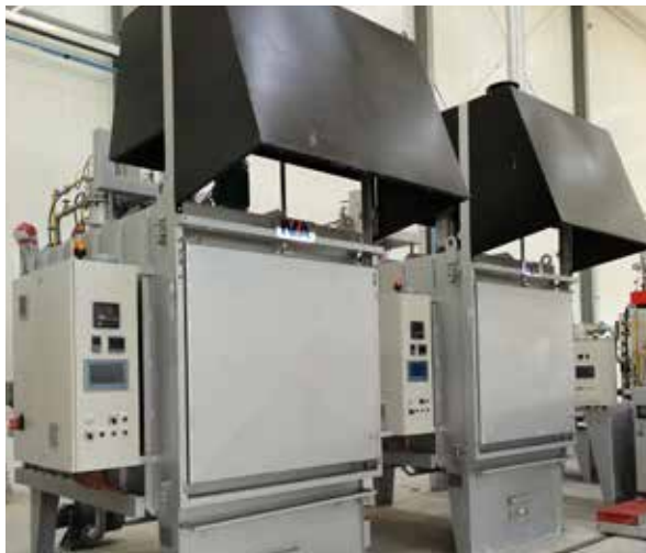
回火炉 Tempering Furnace
